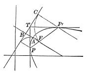
Having constructed either of the diameters, the one, for example through P, draw through T, TB perpendicular to it, and TB will be the directrix of the parabola.
